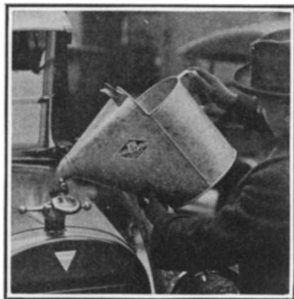
Easy filling of the radiator, without slopping, is achieved with this specially designed bucket
