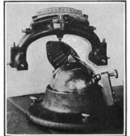
Hardness tester for rapid and serviceable work in the shop
