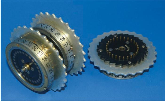
**Fig. 8.2** Example of an electromechanical rotor (from an Enigma)
