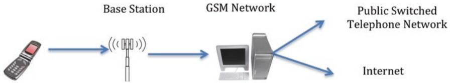
Fig. 12.1 GSM mobile architecture
