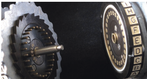
Fig. 10.3 Typical electromechanical rotors. (Wikimedia Commons)
