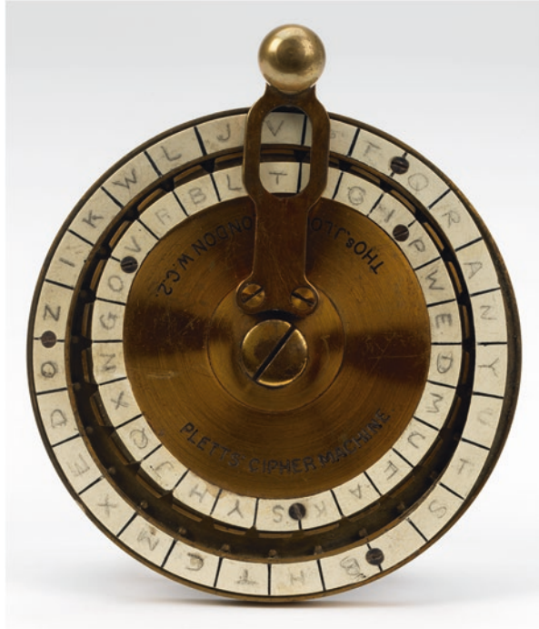
Fig. 4.6 Pletts' cryptograph. (Courtesy of the Imperial War Museum)
