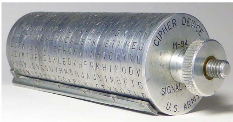
Fig. 10.2 US Army M-94 cipher device (note the third disk from the right is disk #17). (Computer History Museum)
