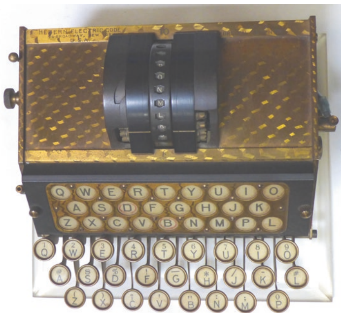
Fig. 10.4 Edward Hebern's original single rotor cipher machine c1921. (Computer History Museum)
