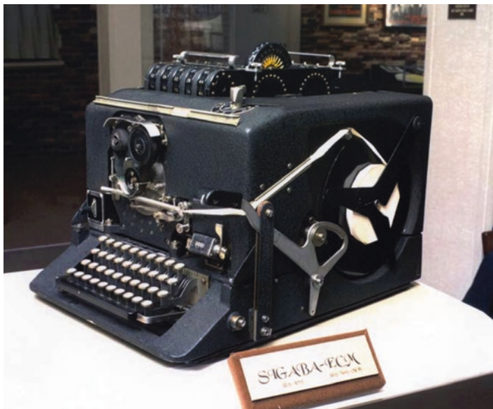
Fig. 17.6 A complete SIGABA machine. (National Cryptologic Museum)
