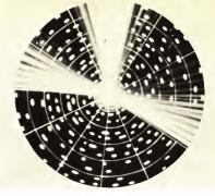
Electronic countermeasures: radar scope jammed by noise from three locations and filled with blips produced by false-target generator
