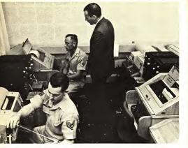
American end of the Moscow-Washington "hot line," with black one-time tape cipher machines standing between the teleprinters
