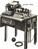
Early Hebern Electric Code Typewriter, using only one rotor
